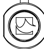
Detail 1:1 bottom rail round hembar 1 1/8" (Ø30mm) cable guided
